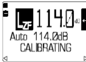
After few moments it will display either FAILED or CALIBRATED. The correct calibration level is  $L_{ZF}=114.0\text{dB}$ .
