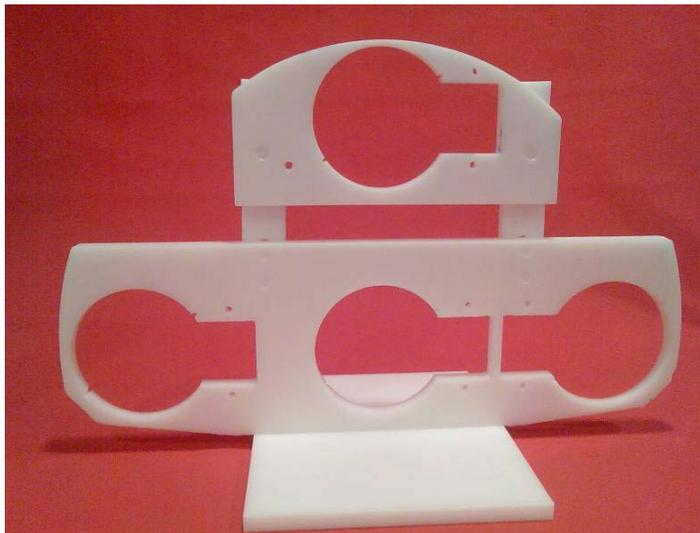
Figure 56. Conventional MRI in the Bore measurement grid
