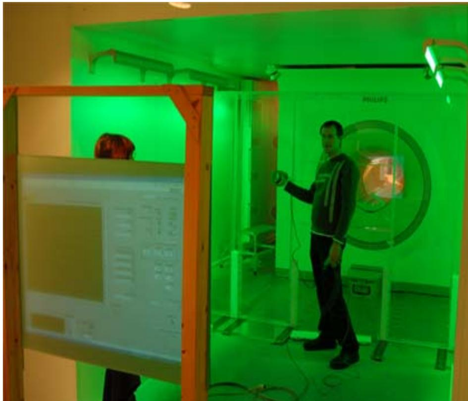
Figure 46. Graphical user interface projected inside the MRI screened room.
